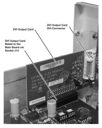
Figure 3 — Output DVI board installation
